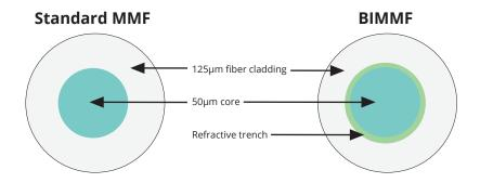
The refractive trench is made of a glass material which has a lower refraction index than the core. This ensures that weakly guided modes are reflected to the core. This way no data is lost when bending the cable in a smaller radius.
