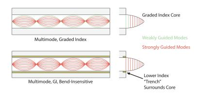
Due to its increased bandwidth, cable lengths, and speed while having a lower weight and total cost of ownership, optical cables have become the preferred cable for numerous applications. Now that bend insensitive optical cables are available (which are less sensitive to data loss), the popularity of optical cables will continue to increase.
