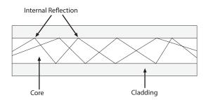
When a cable is bend, the cladding around the core tries to catch the light and guide it along. However, in some situations, such as improper installation or using a cable radius which is too small, the reflection of light in the standard fiber optical cable could no longer be guided by the cladding. This would result in the loss of data. To reduce this loss, many manufacturers are now adding an additional layer to the cable.
